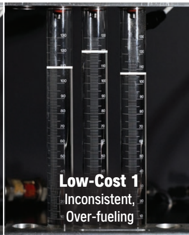
Inconsistent and prone to over-fueling which can cause unburnt fuel to be sent through the exhaust, damaging emissions components
