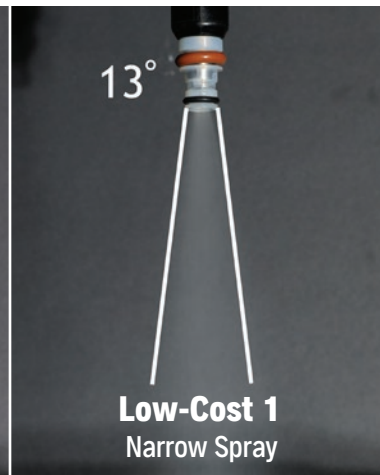
Can result in poor fuel atomization, reducing engine performance and fuel economy
