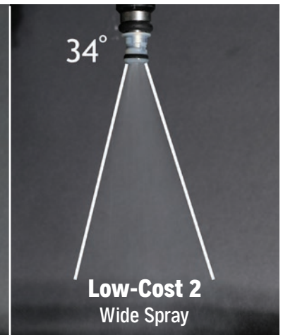
Can result in unburnt fuel dripping down the cylinder wall, washing away oil and damaging the piston rings and cylinder wall
