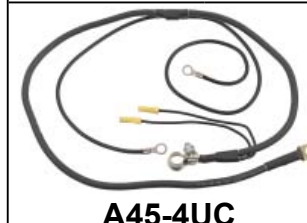
A45-4UC Top Mount Cable F1TZ14301A; F0TZ14301G; BLF290 Battery Cable Configuration: Top Mount - three auxiliary leads Battery Terminal Contains Lead: No Gauge: 4 ga. Length_Dimension: 45" Material: Synthetic Rubber Jacket
